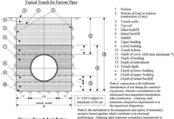
Figure: Trench Installation
